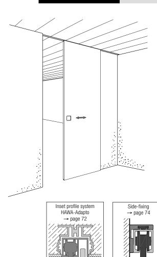
Hardware system for sliding doors weighing up to 80 kg (176 lbs.)
